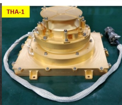
Aditya Solar wind Particle EXperiment - ASPEX instrument onboard Aditya-L1 mission
